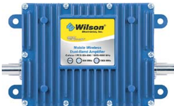
Coupled with an external antenna, this little gizmo — a cell phone amplifier — can give you much more transmitting power.
