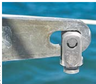
Detail of the broken anchor swivel.
