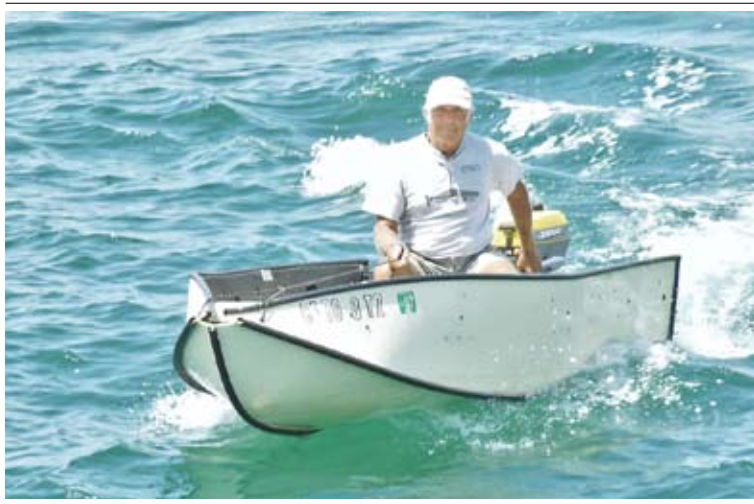
Peter aboard his Port-a-Boat. Although odd-looking, he says it planes easily and is easy to lift aboard by hand. The only drawback is, unlike an inflatable, it doesn't have enough stability to allow you to pull yourself aboard after diving.
