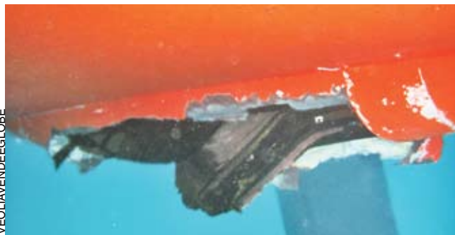
Left, the stump of the keel on 'Veolia Environnement'. Right, an awash shipping container, the likes of which notched three IMOCA 60 'kills.'
