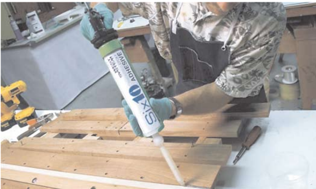
Dispense Six10 Thickened Epoxy Adhesive from any standard caulk gun.
