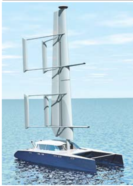
Harbor Wing's test platform and prototype recreational wing rig. Note the biplane air rudders, vertical segmentation and counterweights.
