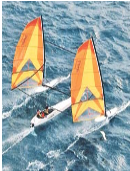
The Hobie Trifoiler, probably the first production biplane rig, transversely divided for low angles of attack.
