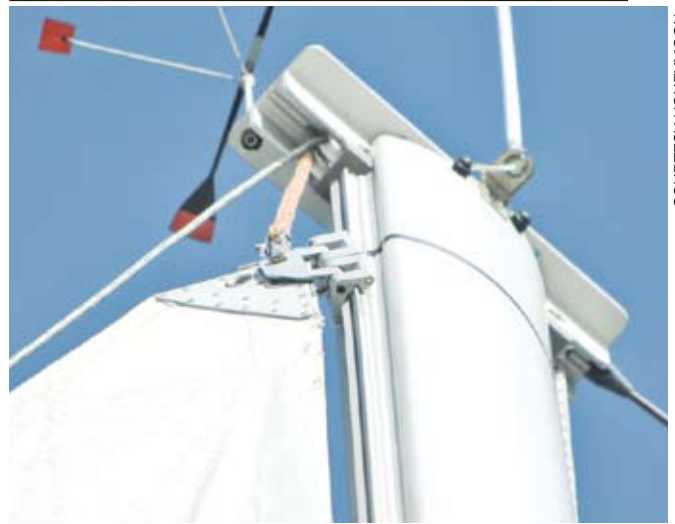
Here's a sight you never want to see far from land: the headboard cars jammed in place at the top of the mast.
