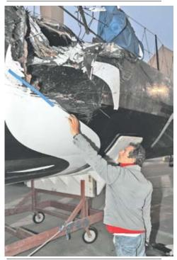
Examining the massive damage to 'Hugo Boss' after it was hit by a fishing boat. Skipper Alex Thompson feels his crew can repair the hull and mast in time for the November 9 start.
