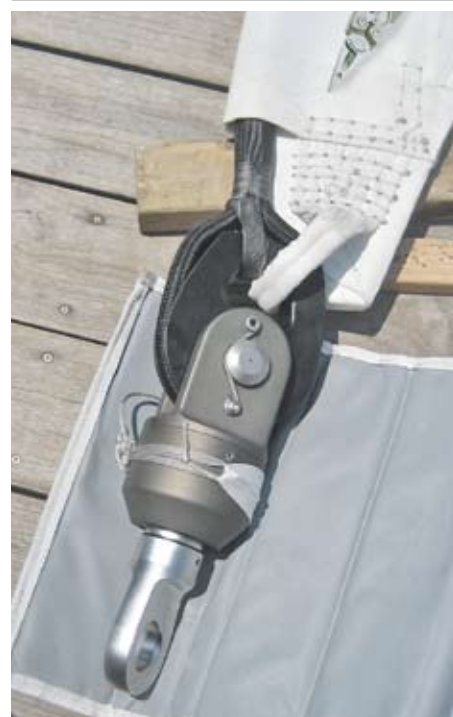
'Speedboat's well-endowed titanium roller-furler swivel measures 12 inches.
