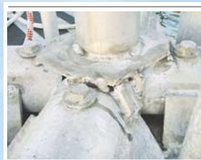
Even though David Vann ended his trip after just two days, he still made it out of the Gate, which is more than many can say. Above, the failed weld.
