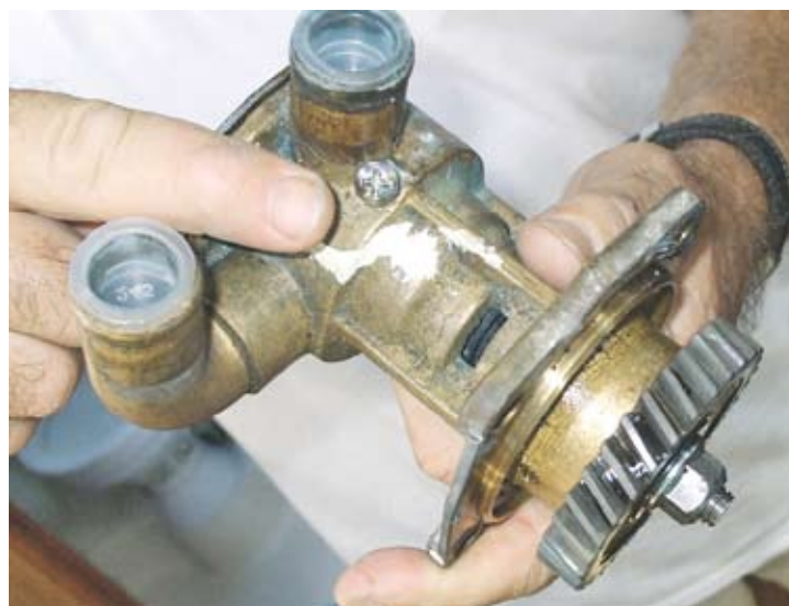
Mike's infamous waterpump: He fixed the leak in the housing with a self-tapping stainless screw dipped in 5200.
