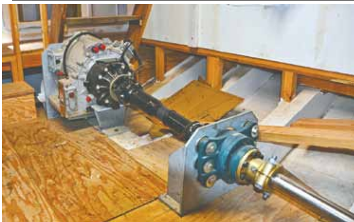
Combining the old with the new, the 'Matthew Turner' has twin 200 kilowatt electric motors, translating to 265 horsepower at each of its screws.
