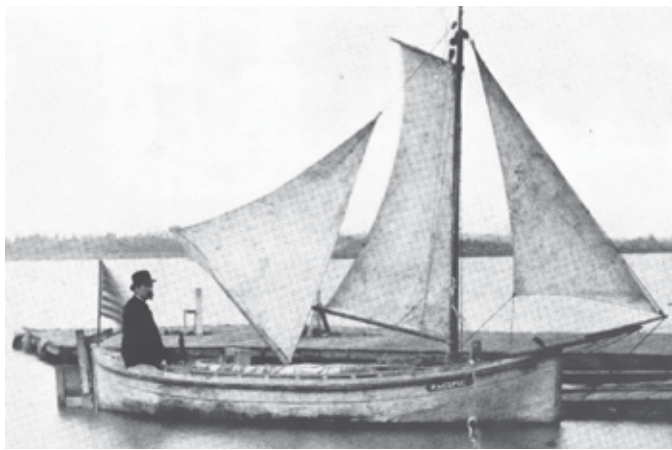
In 1882 Bernard Gilboy made it 7,000 miles across the Pacific on this tiny schooner. He used this jury rig after losing the mainmast.
