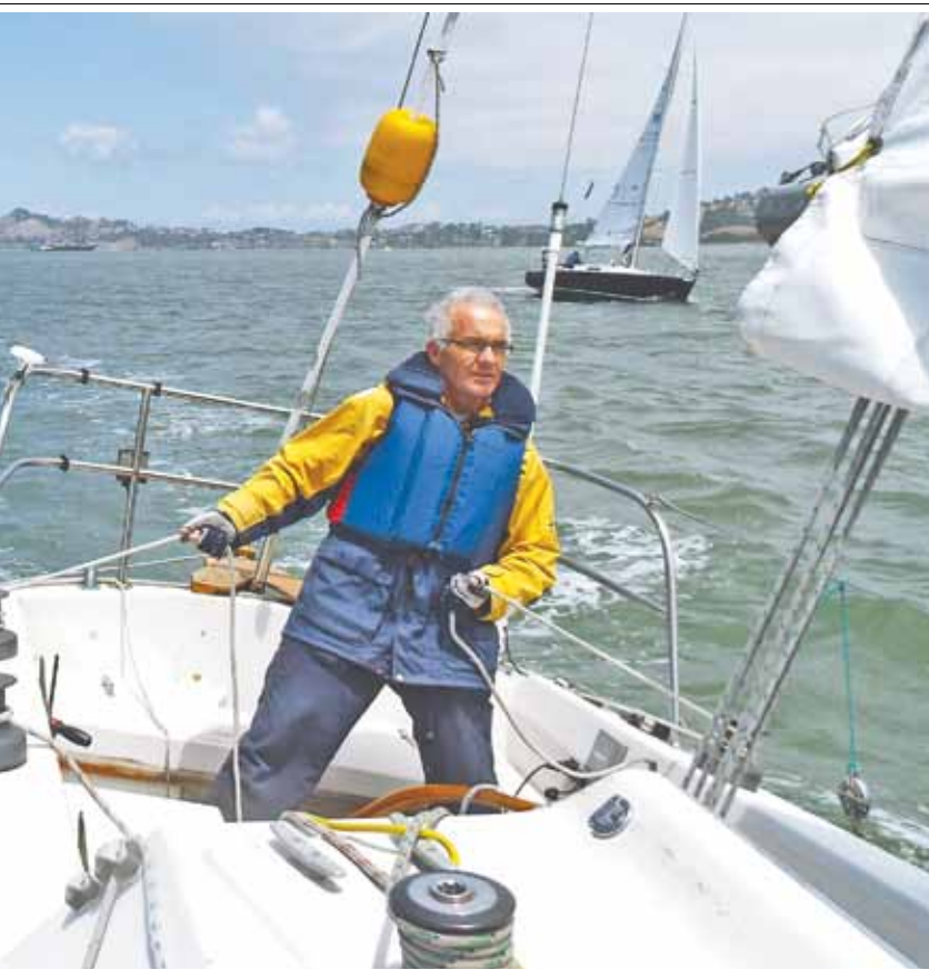
A singlehander tests his emergency rudder setup while racing on the Bay. How effective is your e-rudder? You won't know until you try it.
