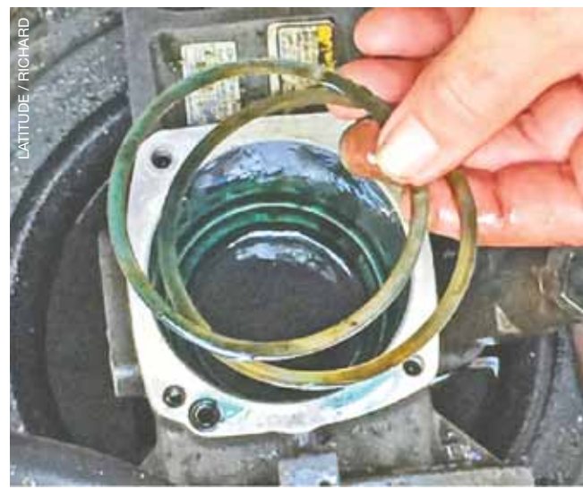
With the clutch assembly tightened down, the shims would come out of alignment, preventing the assembly from fitting into its hole.
