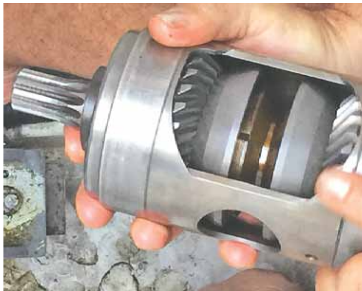
The cone clutch assembly. The bronze-colored thing in the middle of the assembly is the cone drive that can wear out.
