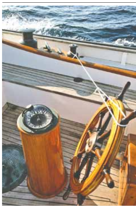
Spread: 'Mayan' ghosts along in SoCal waters. Inset: Prior to installing a modern mechanical unit, the Vrolyks used this elegantly simple, old-school 'autopilot' technique.
