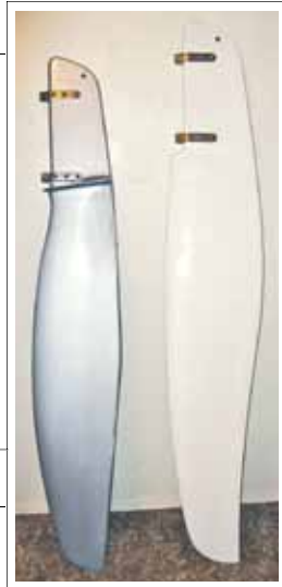
Patrick's new rudder is on the right; the Melges rudder is on the left.
