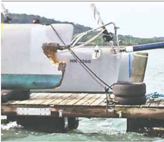
Spread and above: The notch taken out of 'Lakota's starboard ama should be easily repairable. But we can only imagine what would have happened if she'd been traveling at the record-setting speeds she is capable of. Right inset: Wayward containers are a terror to navigation worldwide. In 2011 when the 774-ft 'Rena' slammed into a New Zealand reef, 900 containers went adrift.
