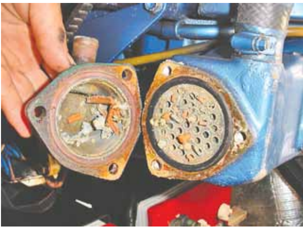
When little rubber fins break off an impeller or zincs break into bits, all that debris often ends up clogging your heat exchanger.
