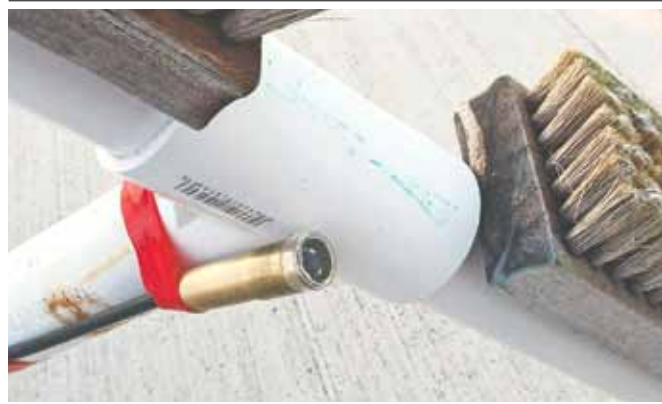
The brush that sees, via an inexpensive waterproof inspection camera on the brush head. Real-time display options are still experimental.
