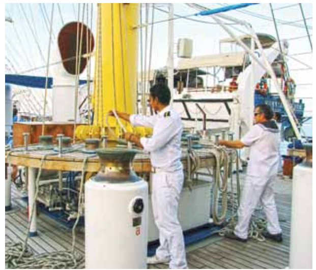
It takes a 100-person crew to run the 'Royal Clipper,' but motorized yardarm furlers lessen the sail-handling workload substantially.
