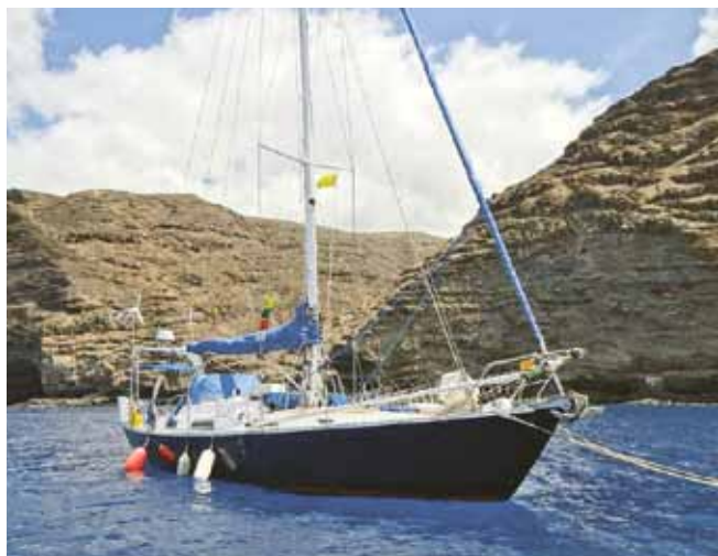
Equipped with solar panels, a wind generator, a windvane steering device, this cutter-rigged cruiser was well-prepared and reliable.
