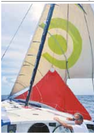
The 'MACIF' crew saved their boom to set up a jury rig.
