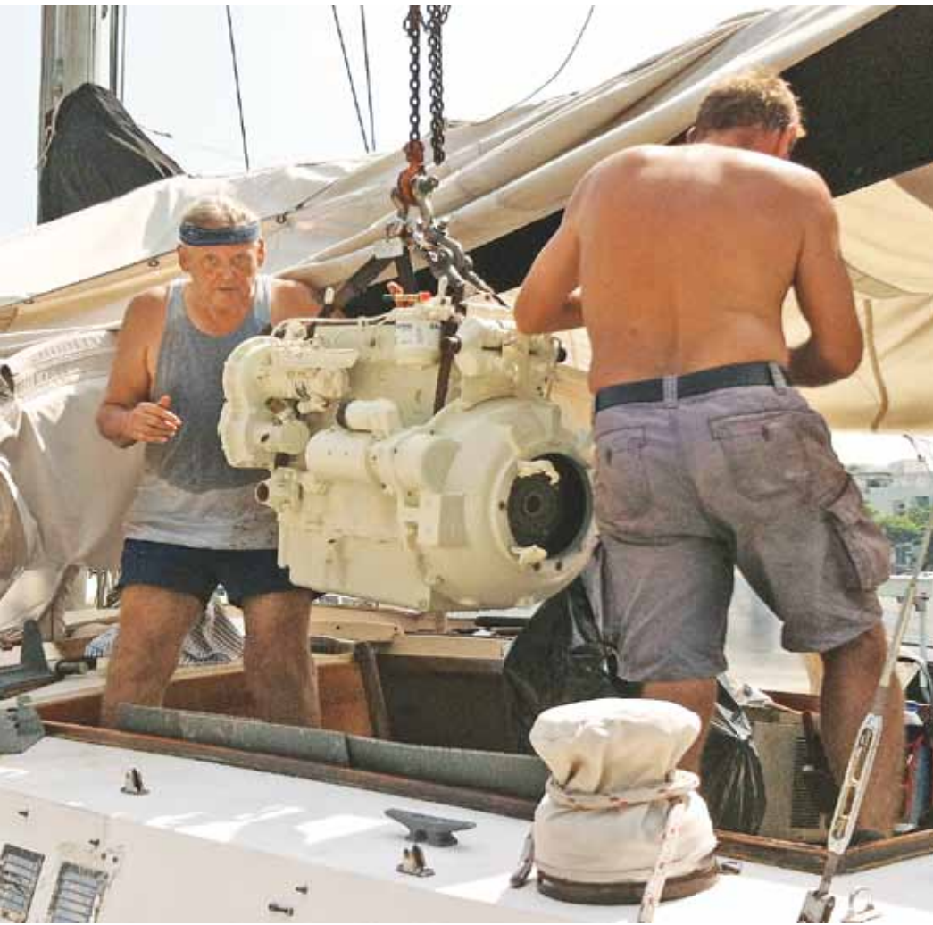
Henry and Mark work to get the rebuilt engine into the engine room. As they had only half an inch to spare, it was a painstaking job.
