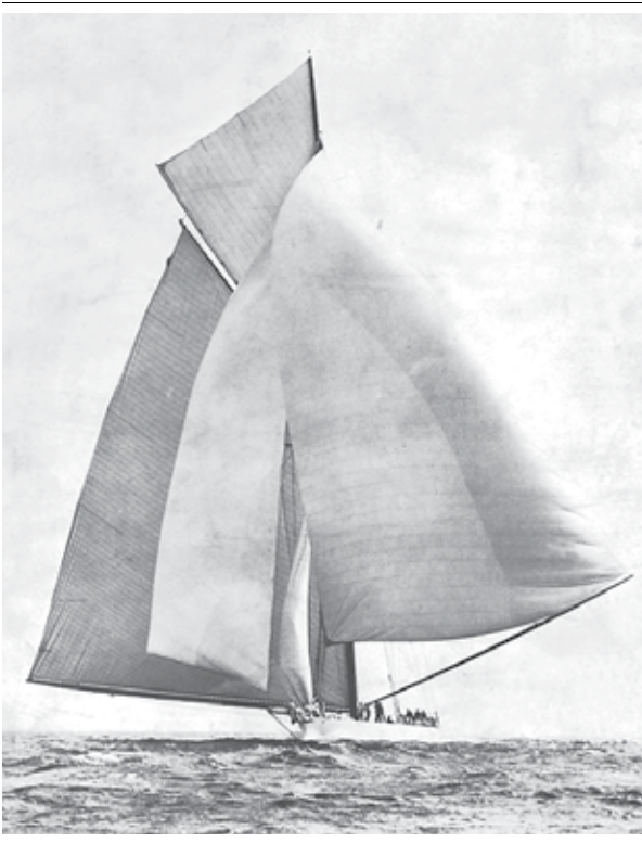
Rigged with a freakish amount of sail, 'Reliance' (202-ft LOA) was the greatest anomaly of the Cup's early years.
