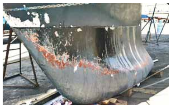
The keel came loose from the pounding on the beach.
