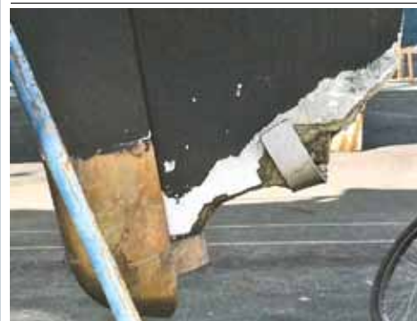
The rudder was also severely damaged.
