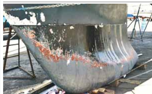
The keel came loose from the pounding on the beach.
