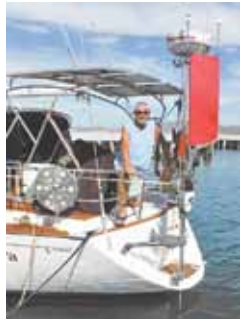
Joel on SV Compañera, a Tartan 3800, in La Paz, Mexico. Hydrovane mounted off-center to preserve the swim platform.
