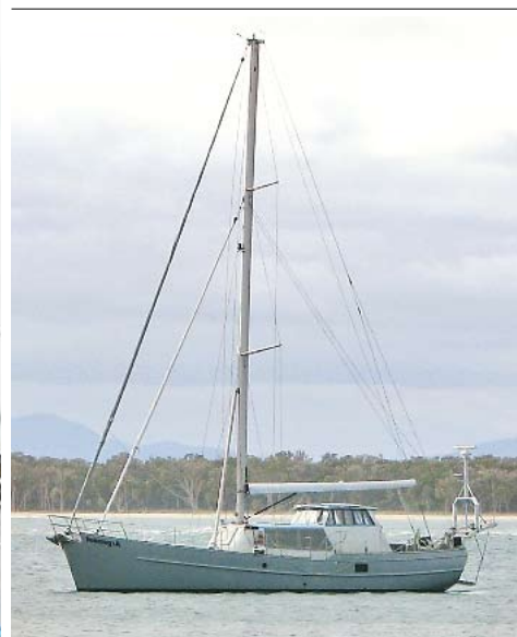
'Argonaut' has a steel hull and deck, and an aluminum house. Rice's family wonder if she may still be afloat in Indonesia.
