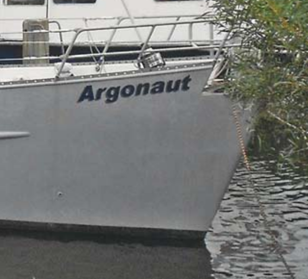
'Argonaut' has a steel hull and deck, and an aluminum house. Rice's family wonder if she may still be afloat in Indonesia.
