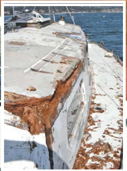
Barry took bucket-loads of rot out of this 53-year-old woody.
