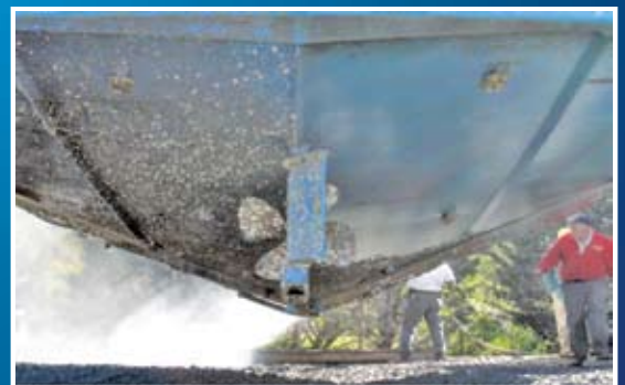
Left: Leading conventional antifouling Right: Pacifica Plus, 12 months Chesapeake Bay
