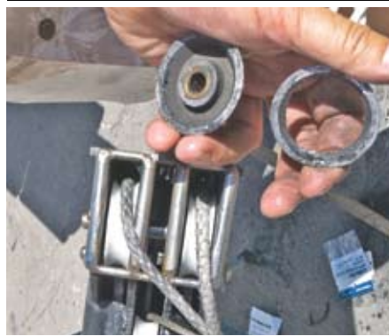
Out with the destroyed aluminum sheaves, and in with the new nylon ones. And all rope halyards, too!
