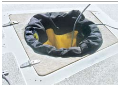
Lee's dry bag spinnaker launcher at the ready to launch (left) and receive (above).
