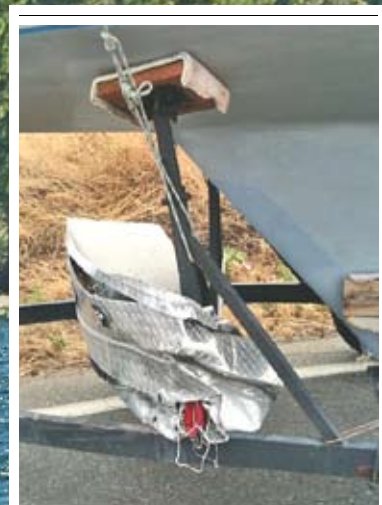
The impact wadded up the trailer box.
