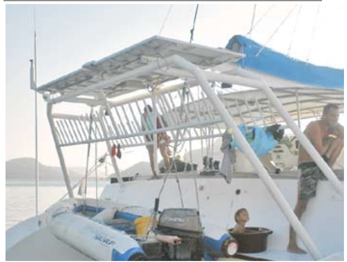
The aluminum structure on the catamaran 'Planet Surf' sort of looked like a giant cheese grater with solar panels on the top.
