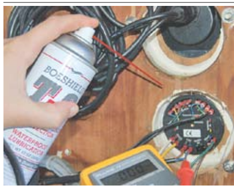
Spray-on protectants, such as Boeshield T-9, are easy and effective ways to prevent corrosion.
