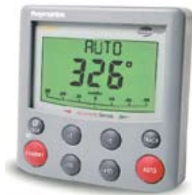
Autopilot head/control units are often the sources of problems, usually due to condensation or corrosion.
