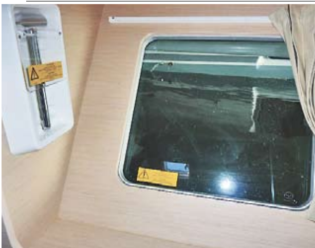
New Lagoon cats come complete with fixed escape hatches — and 'Break Glass In Case Of Emergency' hammers.
