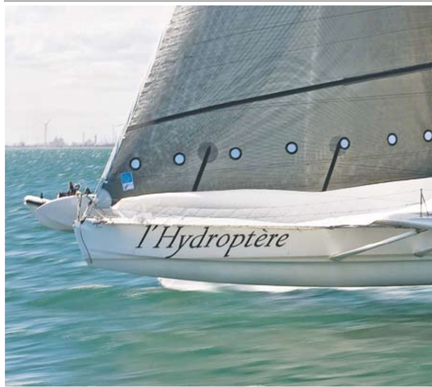
The 60-ft French foiler 'l'Hydroptère' hit 61 knots — a tick over 70 mph — before pitchpoling near Marseilles.
