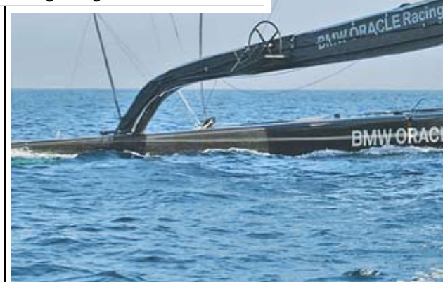
Right before we went to press, BMW Oracle Racing announced they'd be breaking down camp in San Diego and heading for Valencia, but not before putting in a few weeks of testing on their new hard wing sail. Spread, the massive wing gets put through its paces off San Diego. Inset, the two-element wing is 180 feet tall; see the sailor climbing the rig for a sense of scale.
