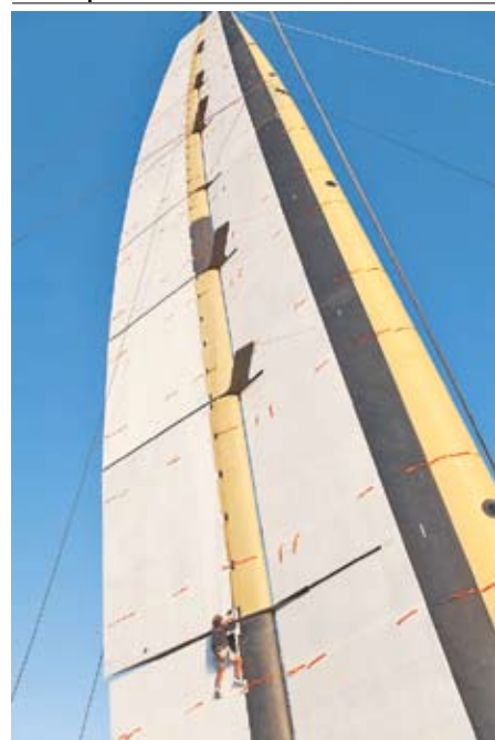
Right before we went to press, BMW Oracle Racing announced they'd be breaking down camp in San Diego and heading for Valencia, but not before putting in a few weeks of testing on their new hard wing sail. Spread, the massive wing gets put through its paces off San Diego. Inset, the two-element wing is 180 feet tall; see the sailor climbing the rig for a sense of scale.
