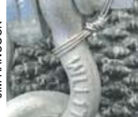
A proper 'mousing' job on a shackle.
