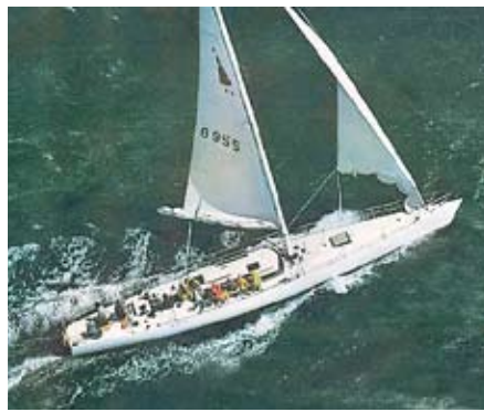
Bill Lee's 67-ft 'Merlin', the original ultralight sled, has been raced hard for over 300,000 miles without a keel failure.
