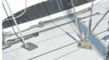
New aft swept spreaders get new chainplates. Next stop Hawaii.
