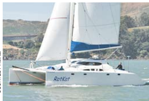
Lightweight composite construction and a rotating mast mean 'RotKat' is capable of very high speeds.
