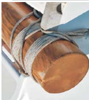
'Rere's beam lashings.
