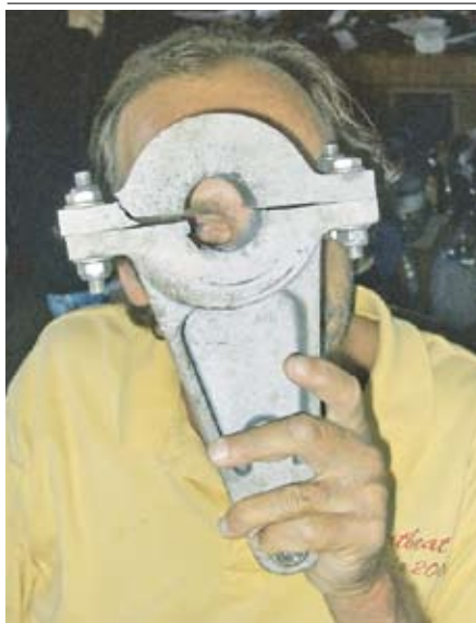
Looking a lot like an unlicensed optometrist, Bill Lilly holds up 'Moontide's' rudder collar so that you can see where the casting failed.
