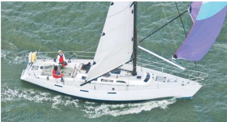
'Punk Dolphin's two-pole arrangement. To jibe: lazy pole up, crank in the old sheet/new guy, ease out the old guy/new sheet — and lower the 'old' pole end to the deck. Couldn't be easier.
