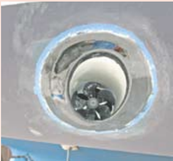
Installing a new bow thruster and teak decks on a Jeanneau.
