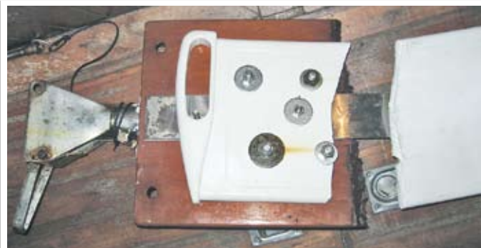
Fix #2 incorporated the centerboard from a Walker Bay dinghy. It lasted five days before snapping in two.
