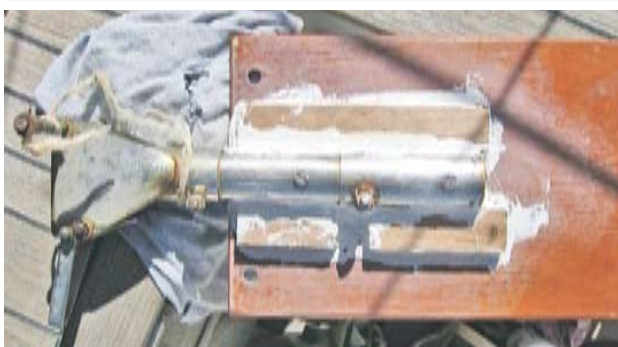
Short-lived fix #1: The centerboard was bolted and epoxied onto the water paddle shaft — which a collision had weakened.
