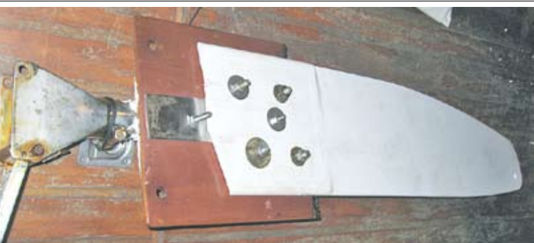
Fix #3, using the undamaged lower portion of the centerboard, lasted for the remainder of the trip.
