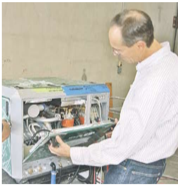
Founder Kevin Alston reveals the guts of an OSSA Powerlite 240-volt DC generator, which requires minimal maintenance.
