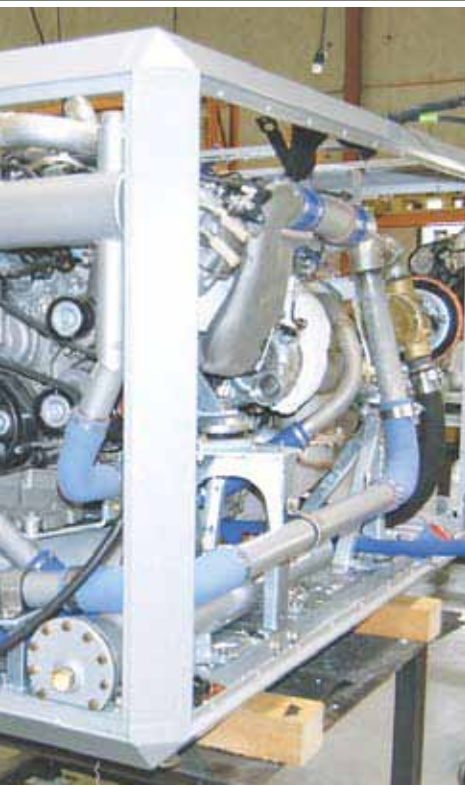
In the Union City plant, craftsmen inspect the workings of a 200-kW generator which will soon be installed on a 72-ft poweryacht.
