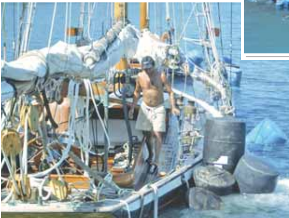
Top to bottom: The Alden schooner lies in 40 feet of water at Meros Island; the long process of positioning the barrels begins while epoxy patches are applied; 'Lord Jim' flops over to starboard before equal balance is achieved; finally, she rises to the surface, high enough so that a gas-powered pump can be mounted.
