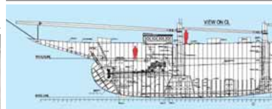
Above, old meets new (note bow thruster) in this modernized side view of William Garden's original design. Inset right, Dutch businessman Ed Kastelein is well known in classic yacht circles for building or rebuilding several large yachts. Spread, 'Atlantic' takes shape in the Netherlands. The new version will be steel, like the original, but welded rather than riveted.
