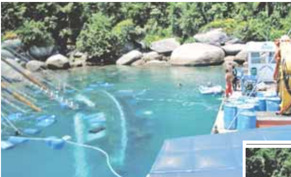
Top to bottom: The Alden schooner lies in 40 feet of water at Meros Island; the long process of positioning the barrels begins while epoxy patches are applied; 'Lord Jim' flops over to starboard before equal balance is achieved; finally, she rises to the surface, high enough so that a gas-powered pump can be mounted.
